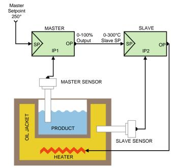
In this example the controlling actuator is a heater, indirectly heating the product via an oil jacket. The maximum input to the slave represents 300°C, thus restricting the jacket temperature. At start-up the master compares the product temperature (ambient) to its setpoint (250°C) and gives 100%. This sets the maximum slave setpoint (300°C), which is compared to the oil temperature (ambient) and the slave requests maximum heater output.
