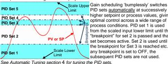
PID sets automatically at successively higher setpoint or process values, giving optimal control across a wide range of process conditions. PID set 1 is used from the scaled input lower limit until the "breakpoint" for set 2 is passed and that set becomes active. Set 2 is used until the breakpoint for Set 3 is reached etc. If any breakpoint is set to OFF, the subsequent PID sets are not used
