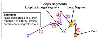
Loop Segment goes back to a specified segment. This action is repeated for the equired number of times (1 to 9999) before the profile continues onwards. More than one Loop Segment can be used, but they must not cross
