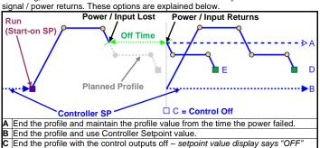
On Recorder versions, option E will always be used if the power / signal is lost for less than the Profile Recovery Time. If the power / signal is lost for more than this time the defined Profile Recovery Method is used.
