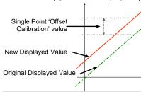
This example shows a positive offset value. E.g. if the process displays 27.8 when it should read 30. an offset of +2.2 would correct the displayed value to 30. The same offset is applied to all values, so at 100.0 the new value would be 102.2.
