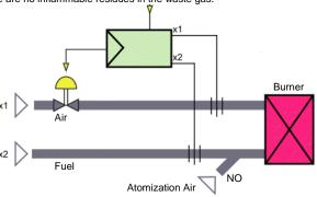
It is normal in this application to display the process value and setpoint as relative values rather than the physical ratio or absolute values. A scaling factor is set such that the displayed value will be 1.00 at the correct stoichiometric ratio for the
