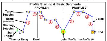
Following a Start Trigger, profiles can start immediately, or if enabled after a delay r at a specified day & time (Recorder only).
