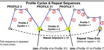
A profile can be made to run itself 1 to 9999 times or continuously using the Profile vcles setting. A profile ending with **Repeat Then End** will run the entire sequence of profiles again 1 to 9999 times or continuously
