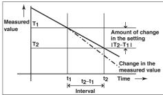
The alarm value of the rate-of-change alarm is set using an absolute value. The interval is derived using the following equation and set using the number of samples.
