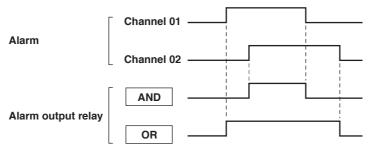
The alarm output relays assigned to AND operation are specified as follows: "I01 (first relay) to lxx (where xx is the relay number)."
