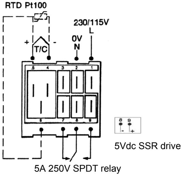
TYPICAL WIRING DIAGRAM FOR SINGLE OUTPUT
