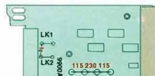
15.2 Supply Voltage Conversion (Plug in links) IMPORTANT - check your installation operating voltage before proceeding. Wrongful conversion could damage this unit.
