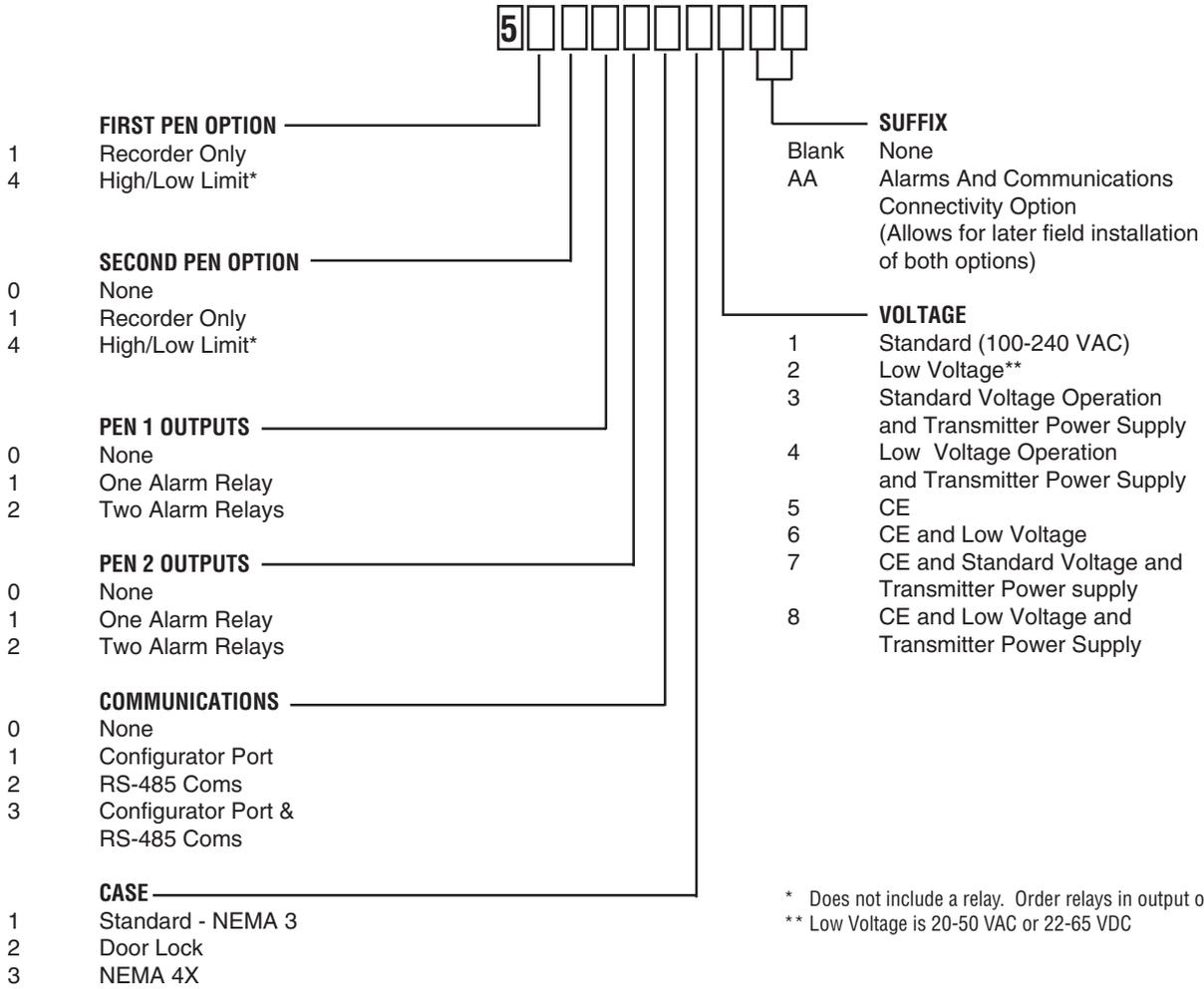
\* Does not include a relay. Order relays in output options.
