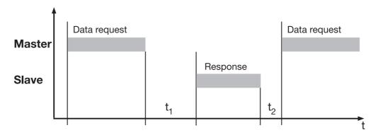
t<sub>1</sub> Internal waiting time of the paperless recorder before checking the data request, and the internal processing time.
