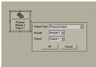
When connected to logic function blocks the specified physical output will switch as the logic driving the output changes state.
