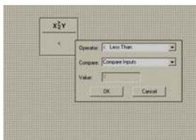
Comparators convert the input level to a percentage of full scale e.g On a logic I/O module input with range of 0 - 24V, an input voltage of 2.4V will be considered to have a value of 10.0 in a comparator block. The compare function allows a greater or a less than comparison with the input. If the comparison is true the block will have a high-state output (1).
