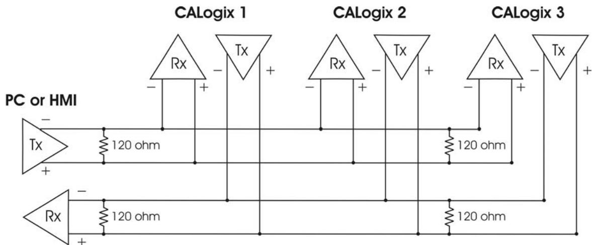
When transmission lines are not transmitting, they remain in an intermediate state which can allow receivers to receive invalid data bits due to electrical noise on the cable. To prevent this bias resistors may be required to force the lines into a known state. Some RS485 interface cards and converters may have bias resistors fitted please check manufacturer's specification and recommendations for use of bias resistors.
