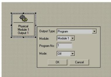
When the input to the block is high (1), the chosen programmer function will be activated.
