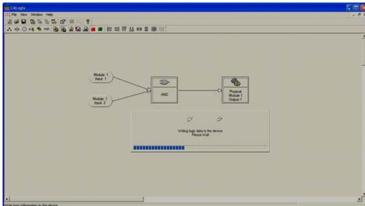
As the program is being written to the controller a progress bar is visible.
