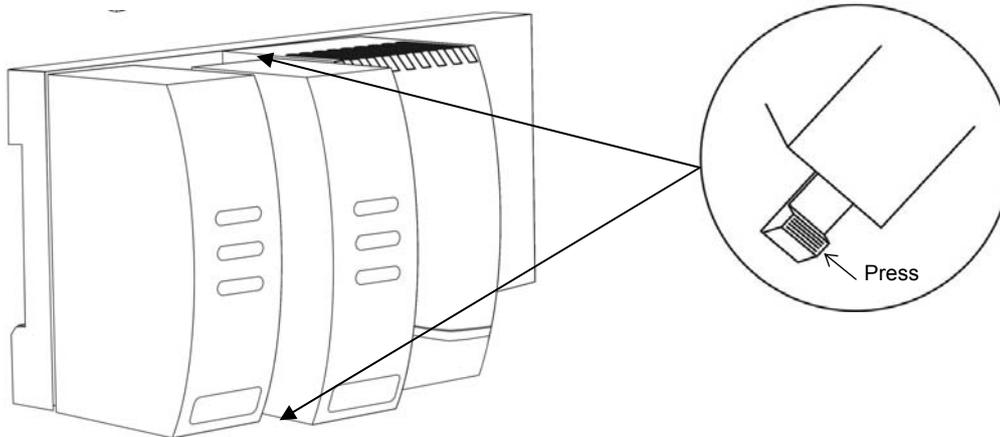
4. Pre-wire connectors and plug into the appropriate modules (we suggest wire markers for identification)
