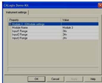
A user-defined label (name) for the module can be entered in the **module name** field, once a label is entered click on the apply button to write the label to the controller. This label will be visible on the controller image in CALogix-sw and will be included when the application is exported to .rtf files. The label can have a maximum of 10 characters
