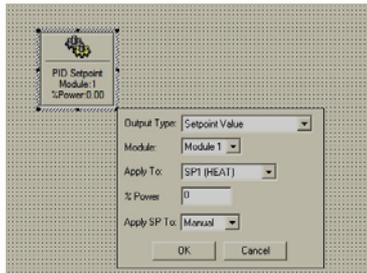
Manual power can be selected to apply to SP1, SP2 or SP3 of a specified module and will operate when input to the block switches from low (0) to high (1) logic state.
