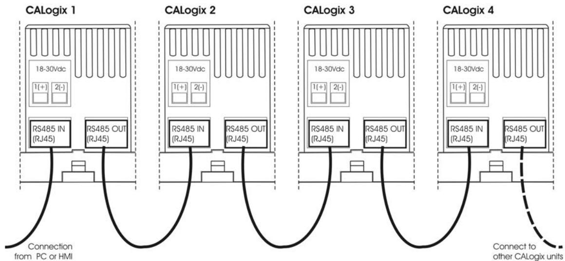
For multiple instrument networks each transmission line must be properly terminated to prevent reflections. 120Ω termination resistors should be fitted between TX+ & TX- and RX+ & RX- at the connection to the PC in addition to the last instrument in the chain. See example below.
