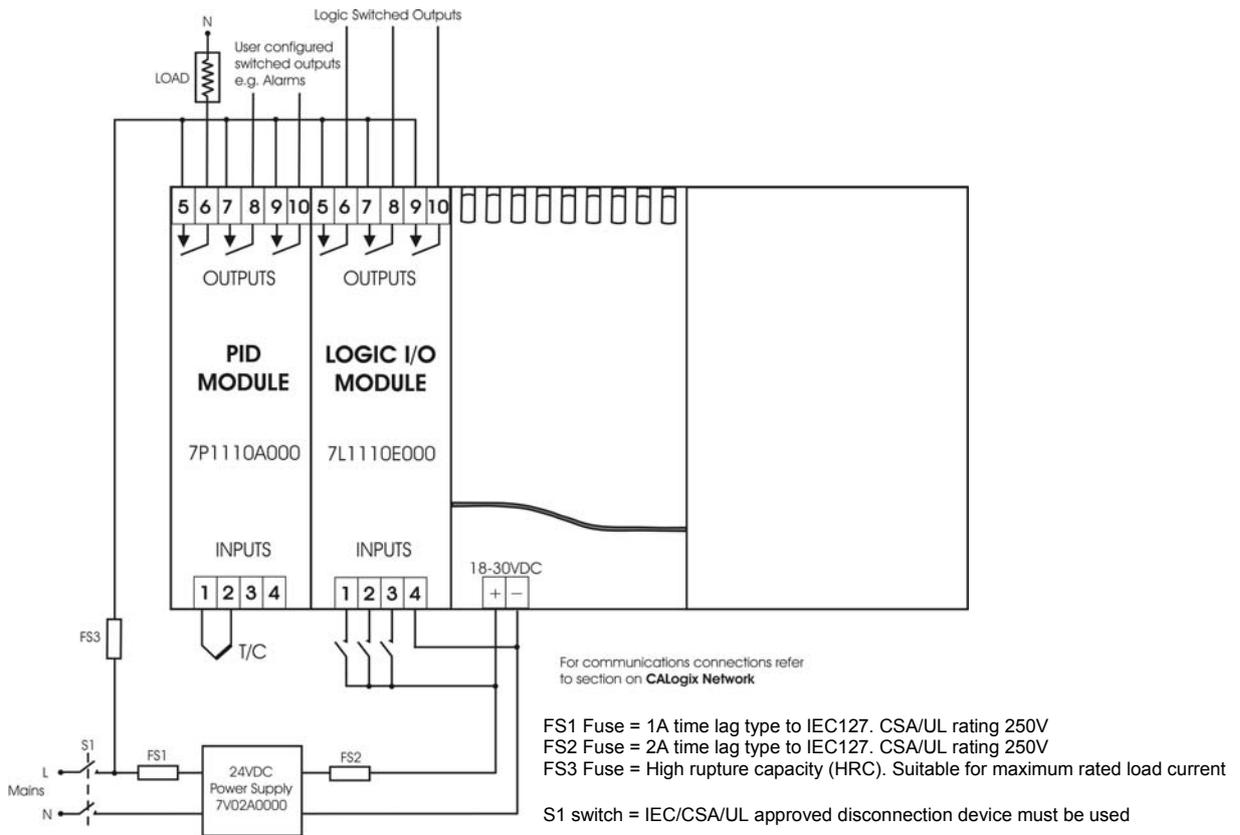
It is strongly recommended that the power supply zero volts and all logic module zero volts are common to prevent ground loops.
