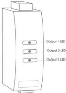
CALogix base-unit has three status LED's to assist with diagnosing problems
