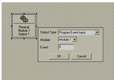
For easy identification it is recommended that you give an event input the same number as the segment in the program. For instance if the EIP segment is 4 then set the event input to number 4 in the logic, This will mean that when the EIP segment is displayed it will appear as EIP4.
