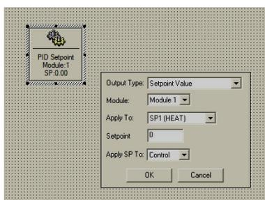
The setpoint change can be selected to apply to SP1, SP2 or SP3 of a specified module.
