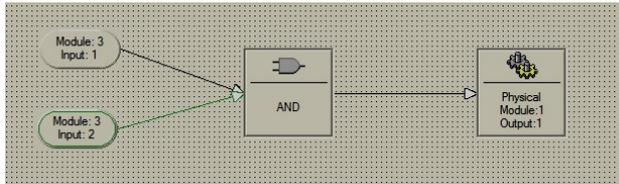
As the output of a function block becomes active (1) a green triangle is shown on the top left corner of the block.
