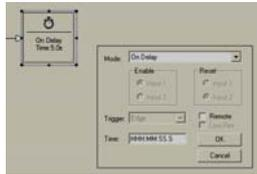
The time settings are entered by clicking on the time required and entering the data in HHH.MM.SS.S format. Once entered click on OK to accept the settings change.
