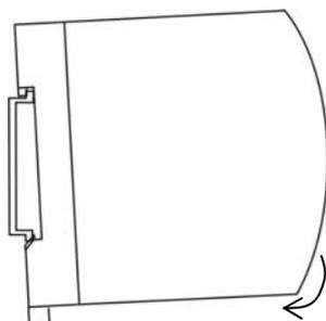
3. Ensuring the input terminals are facing downwards, add the control modules to base unit. Press the top and bottom tabs on the module lightly and ensuring module is kept straight, push to locate in base unit (see diagram below).
