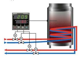
The Oenoreg+ has separate outputs to independently control the Hot and Cold water circuits.
