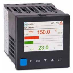
• Modular automation system in a 1/4-DIN (96 x 96mm) format
