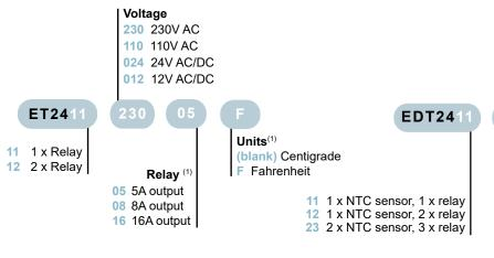
12 12V AC/DC RTC Real-time clock (2) 24V AC/DC SM 9-30Vdc / 7-24Vac Units **Modbus Selection** (blank) Centigrade (blank) Not fitted F Fahrenheit RS Modbus RTU Relay
