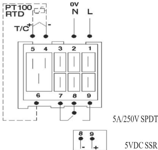
TYPICAL WIRING DIAGRAM FOR SINGLE OUTPUT
